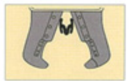
I-beam sheared by shear blades
